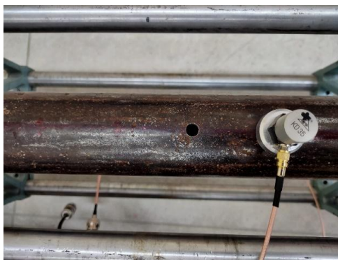
Fig. 4. Photo of a pipeline with a defect of 8 mm
