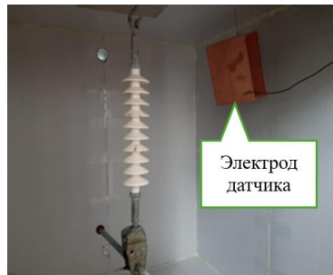
Fig. 1. Geometry of the 3D model of the LK70/35 insulator and its photograph with a capacitive sensor electrode in the "fog" chamber
