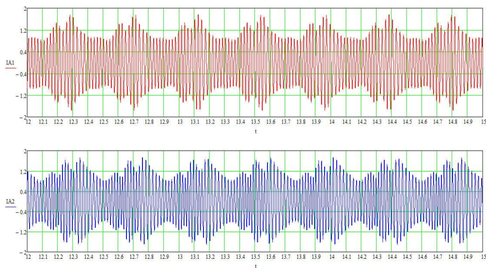
Fig. 8. Results of modeling: D_{n1}=0,002 ; D_{n2}=0,01 ; K_{\omega 1}=50 ; K_{\omega 2}=50 ; \omega_{r01}=1,04 ; \omega_{r02}=0,94 . IA1, IA2 are currents of the parallel-running generators
